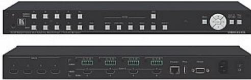
VSM-4x4A is a 4x4 seamless matrix switcher that can also be used as a video wall driver (2x2 or 1x4) or dual and quad multi-viewers. The unit enables switching between inputs with a clean video cut (frame-to-frame switching with no glitches). It supports HDMI resolutions with deep color, up to eight channels of audio and includes per-port HDCP and EDID settings
